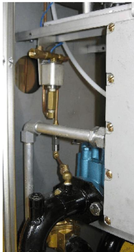
**Fig. 5: Injection Point for HS section of HS/LS-2-DYE / Point d'injection de la section HS du HS/LS-2-DYE**
