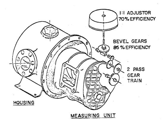
EXPLODED VIEW - METER WITH DB GEAR TRAIN
