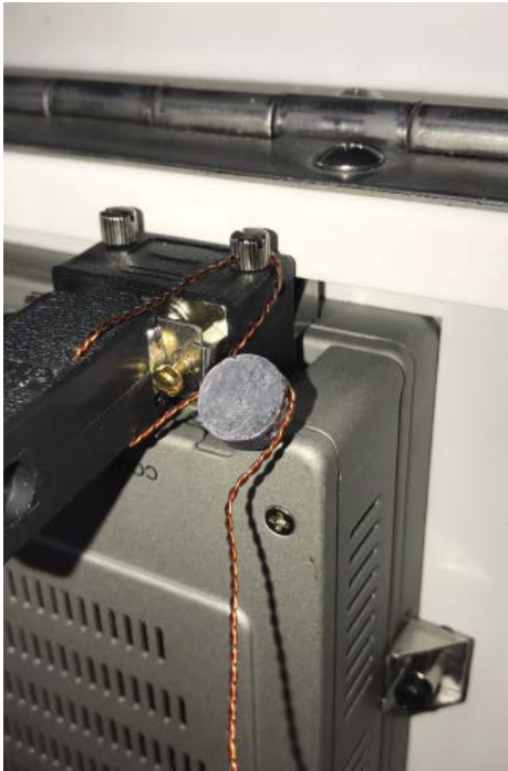
Figure 4: Card lock and MCR-09 register connection sealing / Scellage de la connexion entre le card lock et le registre MCR-09
