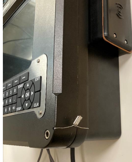
Figure 16: Seal on the enclosure (MultiLoad III EX) | le sceau sur le couvercle (MultiLoad III EX)
