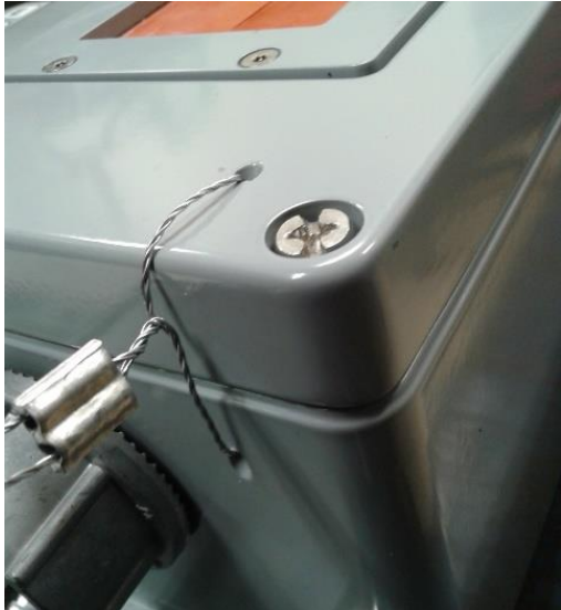
Figure 15: Seal on the enclosure (MultiLoad II DIV-2) | le sceau sur le couvercle (MultiLoad II DIV-2)
