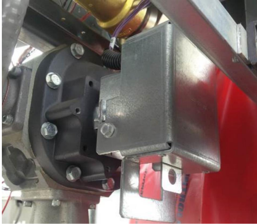
Fig. 4 Optional factory installed security cover for M5 equipped models for owner supplied lock. Sealing under the cover is the same as shown in Hydraulic structure of High Speed dispensers
