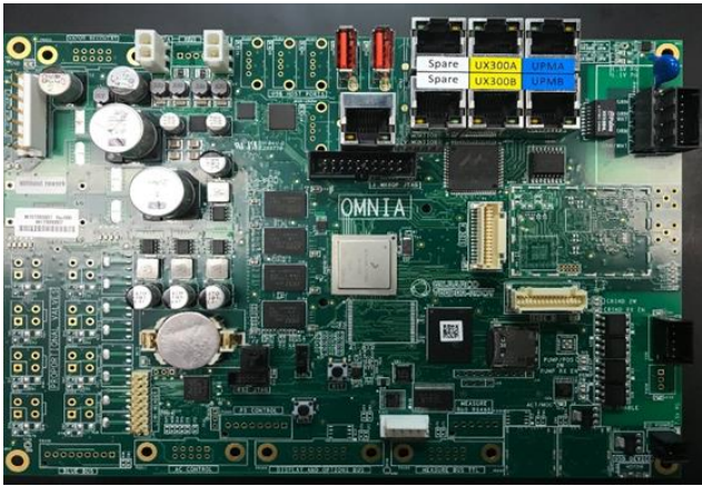
Figure 11: Omnia board, M15758Axxx model (front) | Carte Omnia modèle M15758Axxx (vu de face)
