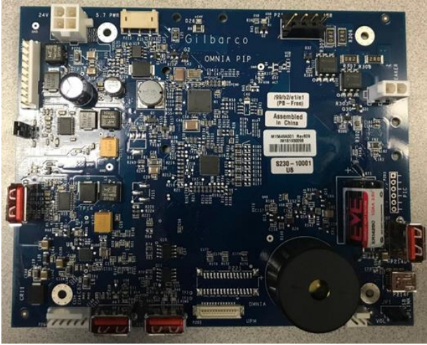
Figure 8 : Omnia board, M15649A001 model (front) | Carte Omnia modèle M15649A001 (vue de face)
