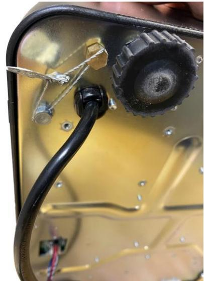
**Typical Sealing UNI-8B and UNI-8P / Scellage typique UNI-8H and UNI-8P**
