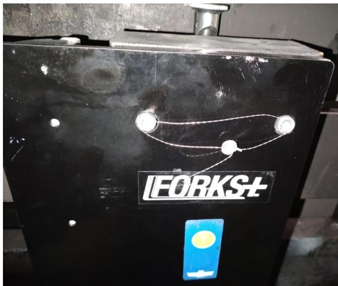
Typical sealing of forks/ Scellage typique des fourches
