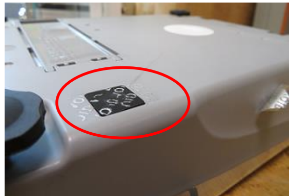
Typical Sealing (circled) / Scellage typique (encerclé)
