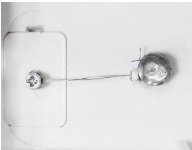
Typical Sealing for TS3X-15, TS5X-15,
