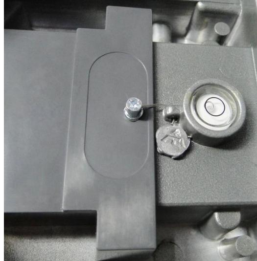
Typical Sealing for TS6X-15, TS6X-30, OS6X-15 and OS6X-30
