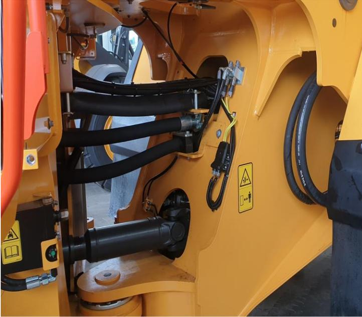
**Typical installation of pressure transducer /
