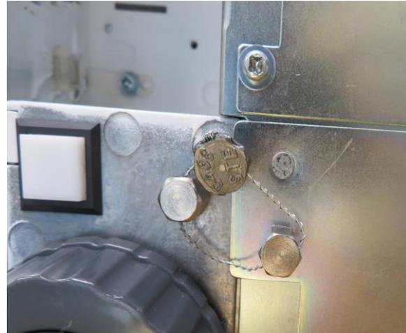
**Typical Sealing for RM-5900x on the calibration switch
