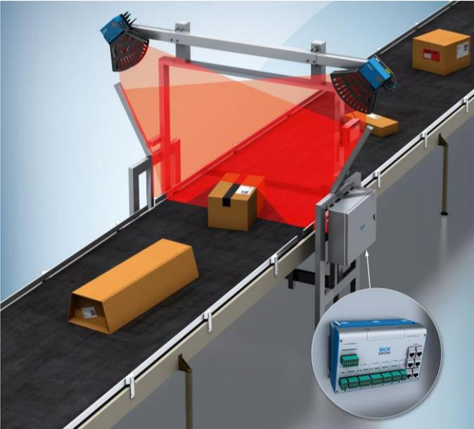
**Typical Dimensioning Arrangement VMS5200 /
