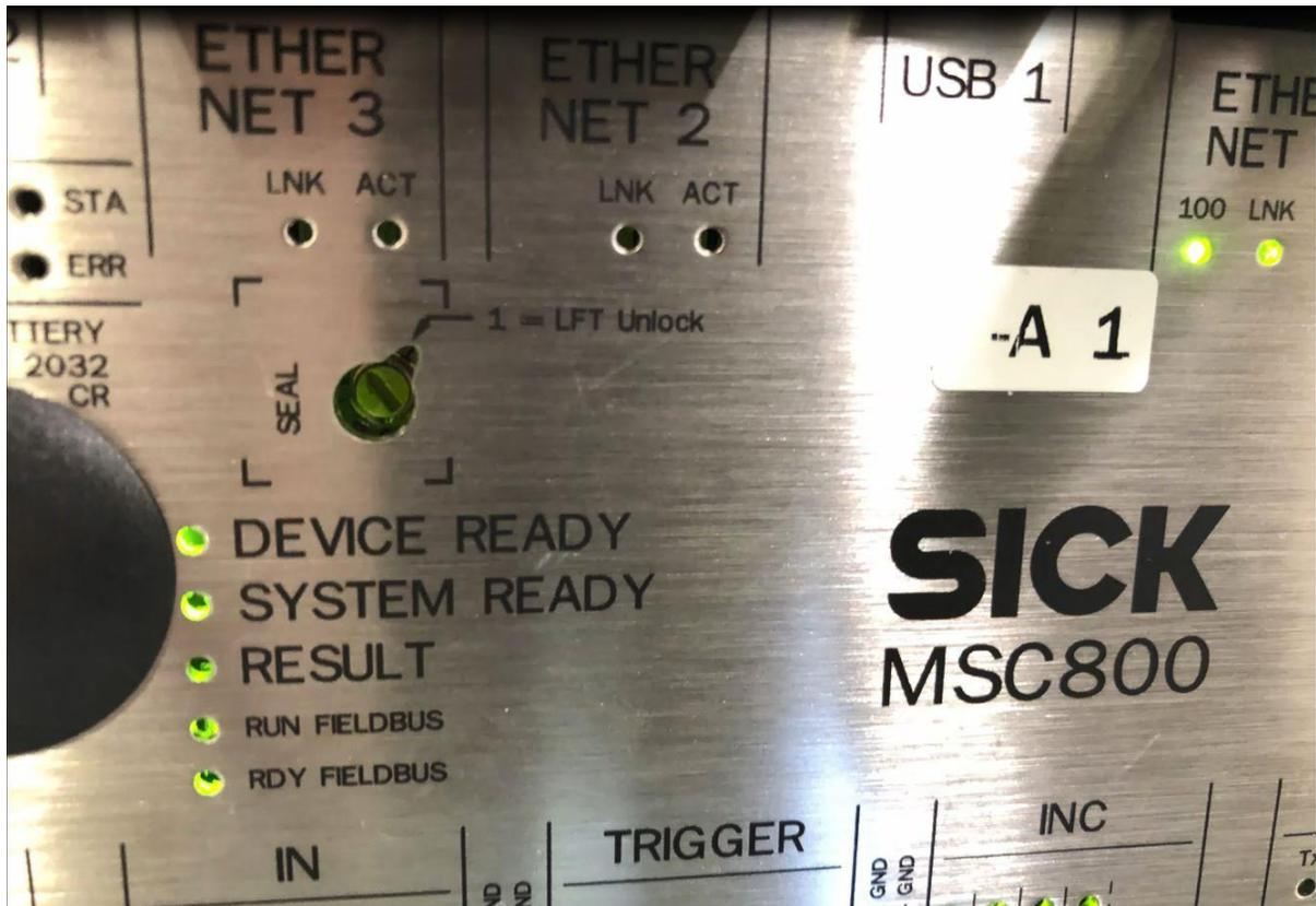
MSC800 controller with location of rotary sealing switch in the sealed position /
