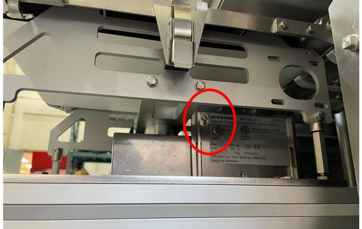
**Location of calibration switch (Configuration B) /
