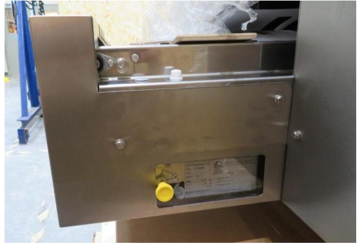
**Location of seal (Configuration A) / Emplacement du scellage (configuration A)**
