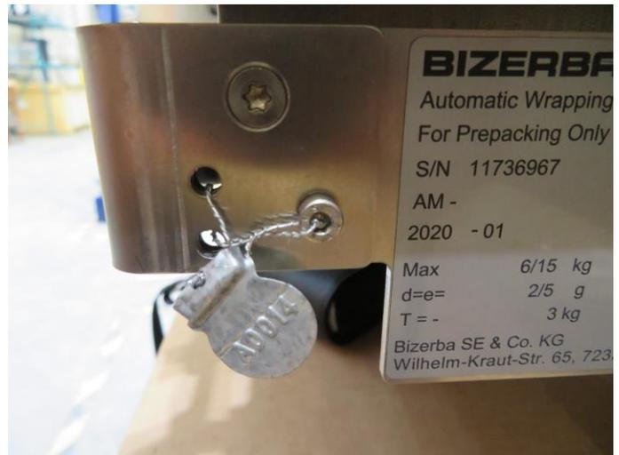
**Typical Sealing (Configuration A) / Scellage typique (configuration A)**
