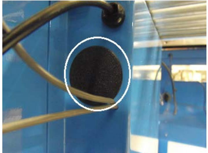
**Typical plug to be sealed by a paper seal (circled) /
