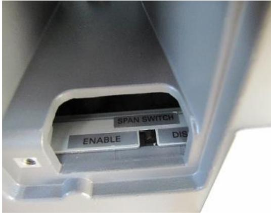
Typical calibration switch access for SM-5300SSP /
