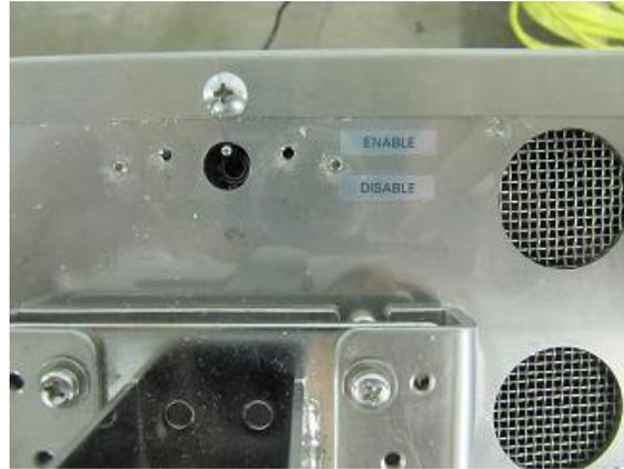
Typical calibration switch access for SM-5300H /
