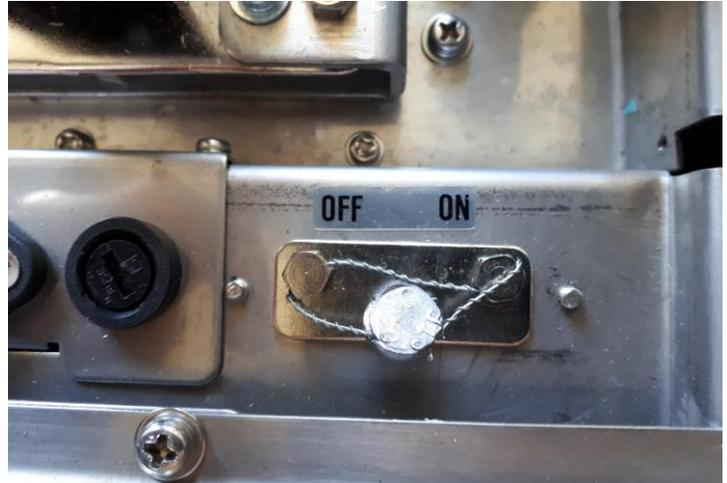
Typical Sealing for RM-5800H on the calibration switch
