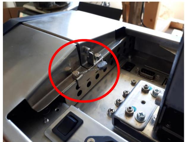
**Typical Sealing for RM-5800H on the housing /
