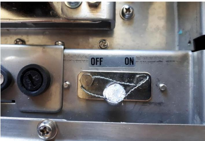
**Typical Sealing for RM-5800H on the calibration switch
