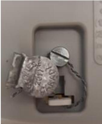
Typical PRyNz sealing on bottom of device/
