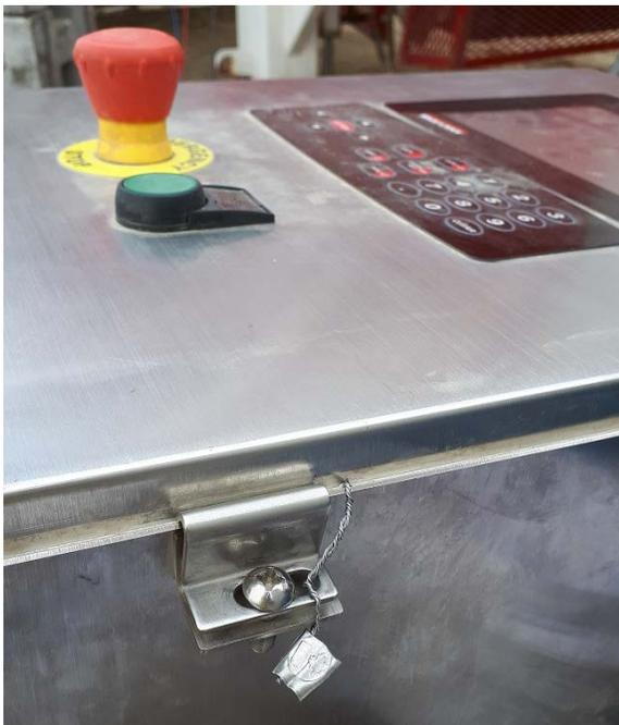
**Sealing of indicator, to prevent access to inclinometer and
