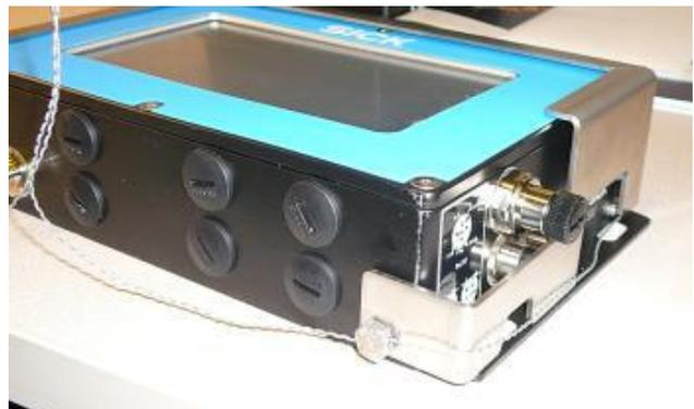
**Typical display sealing (3 drilled-head screws) /
