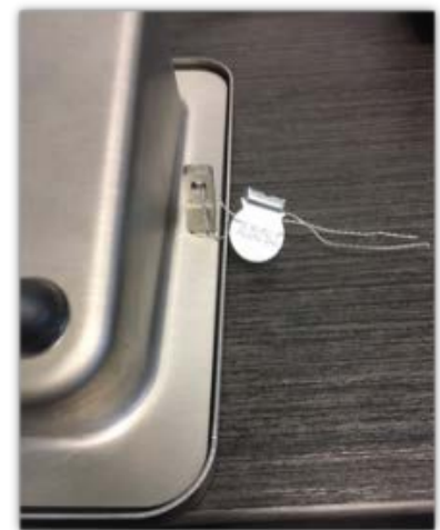
Typical sealing (1 of 2 identical seals) / Scellage typique (1 des 2 scellés identiques)
