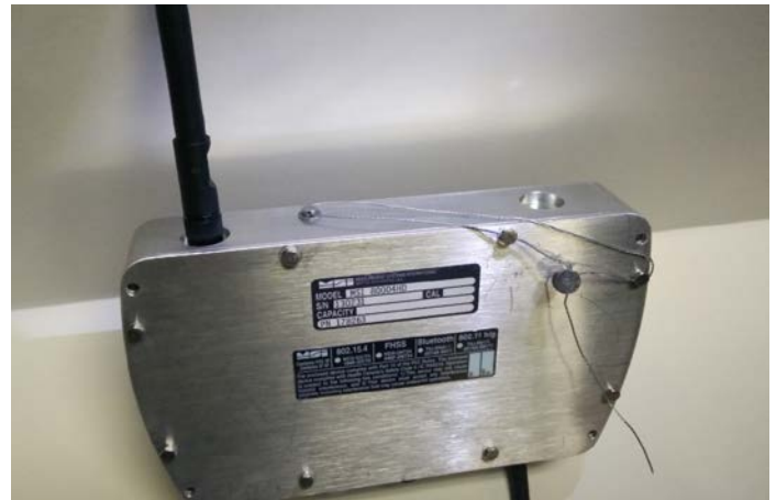
Typical Sealing / Scellage typique
