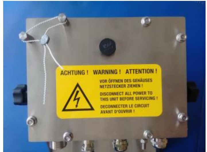
Typical Sealing / Scellage typique
