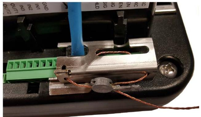
Typical Sealing to prevent access to the internal components /
