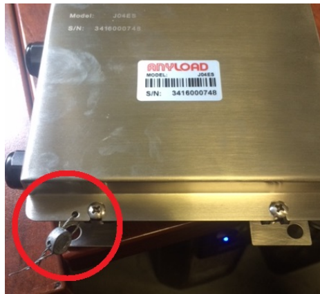
Typical Sealing / Scellage typique
