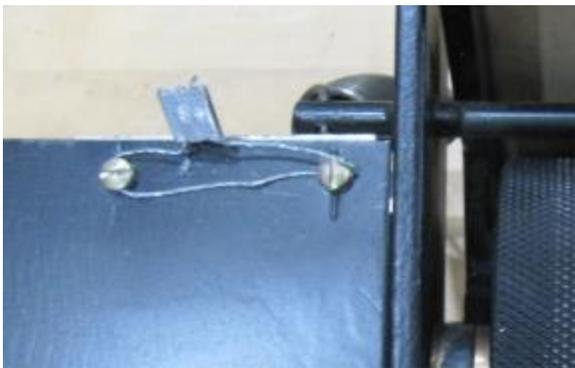
**Typical wire and seal method (display housing, cover plate, and cable connection) /
