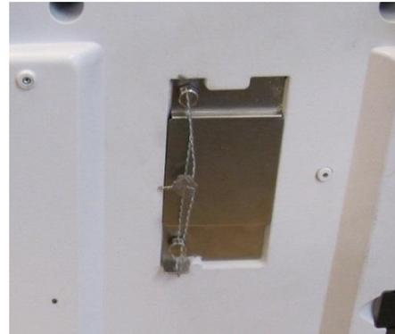
**Typical SD card sealing under the operator's keyboard /
