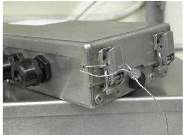
**Sealing of sectional controller model ACC-2000-1A /
