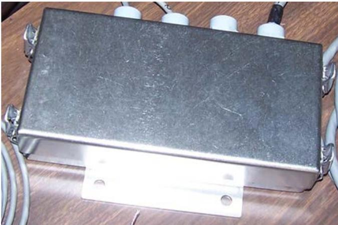
**Typical sectional controller model ACC-2000-1A/
