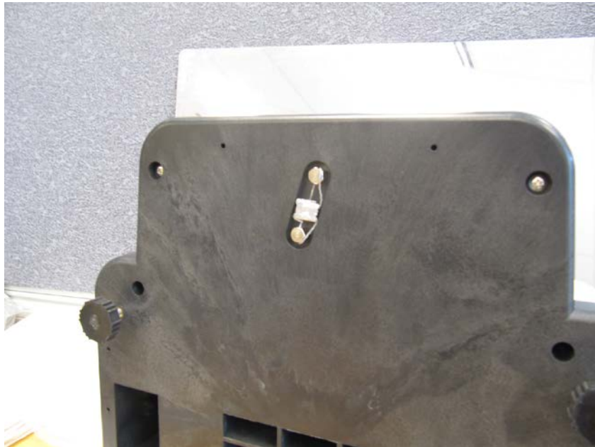
Location of sealing under the scale / Emplacement du scellage en-dessous de la balance
