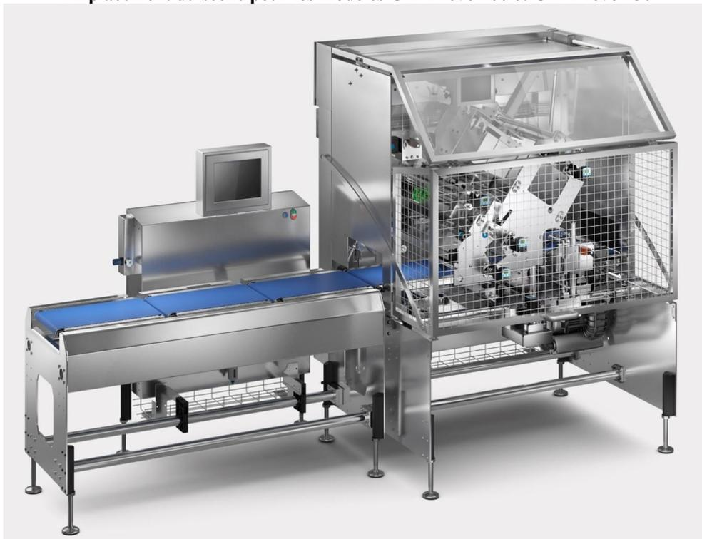
Typical GLM-Ievo coupled to Bizerba F-Wrap "CleanCut" printer /
