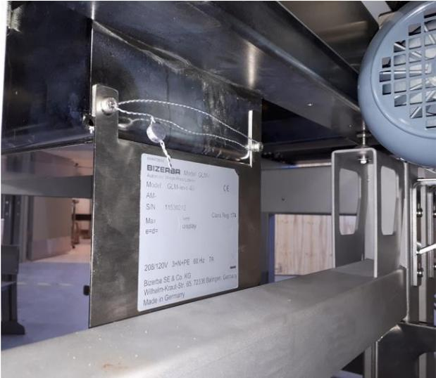
**Typical sealing under the scale of model GLM-Ievo 40 /
