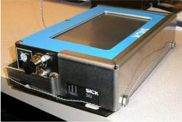
**PARTIE 8 - Photos et dessins (suite)**
