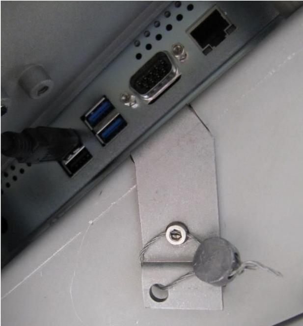
Typical sealing method for model KH II 400-# /
