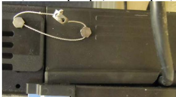
**Typical sealing method for the cable of the modular weighing and load receiving element /
