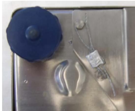
**Typical sealing method for the cable of the modular weighing and load receiving element /
