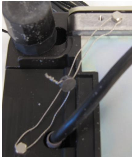
**Typical sealing method for the cable of the modular weighing and load receiving element /**
