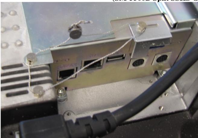
**Typical sealing method for SD memory card and main
