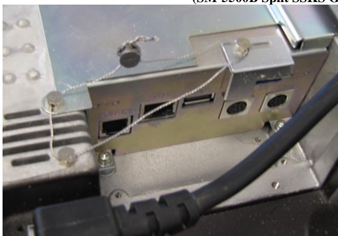
**Typical sealing method for SD memory card and main access plate /**
