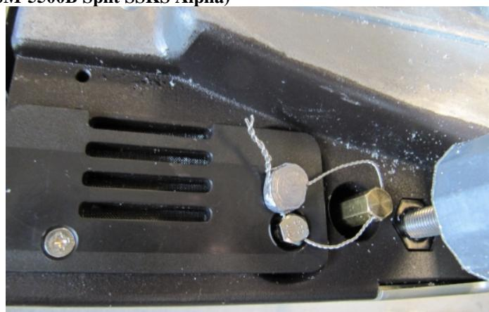
**Typical sealing method for housing access to prevent calibration switch access /**
