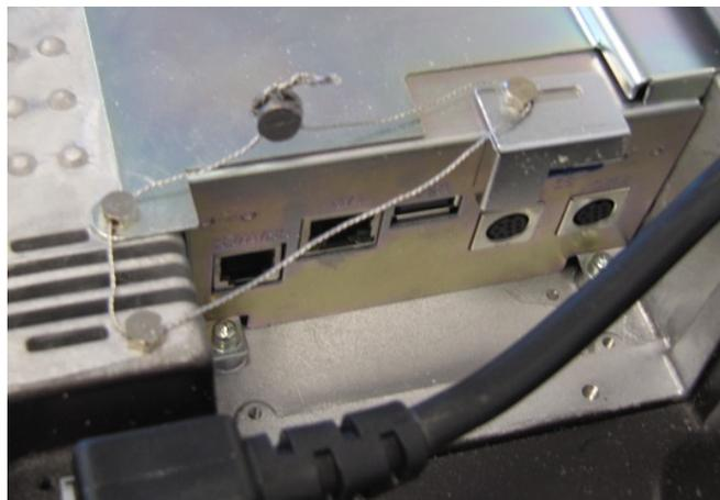
**Typical mandatory seal method for SD memory card and main access plate /
