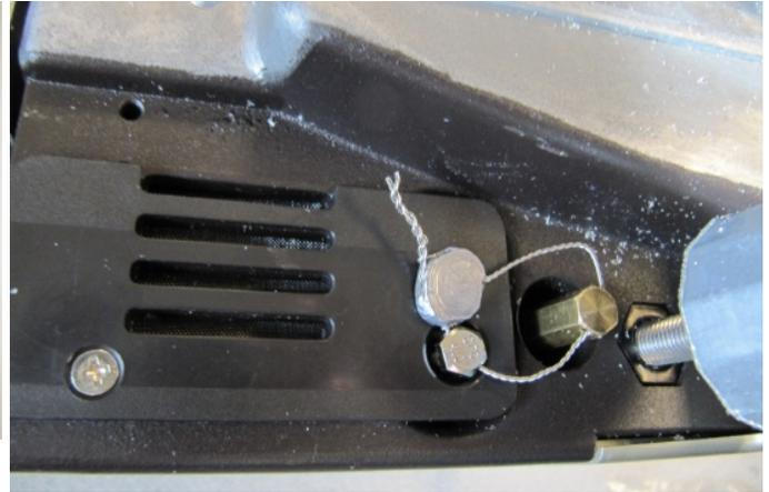
**Typical seal method for housing access to prevent
