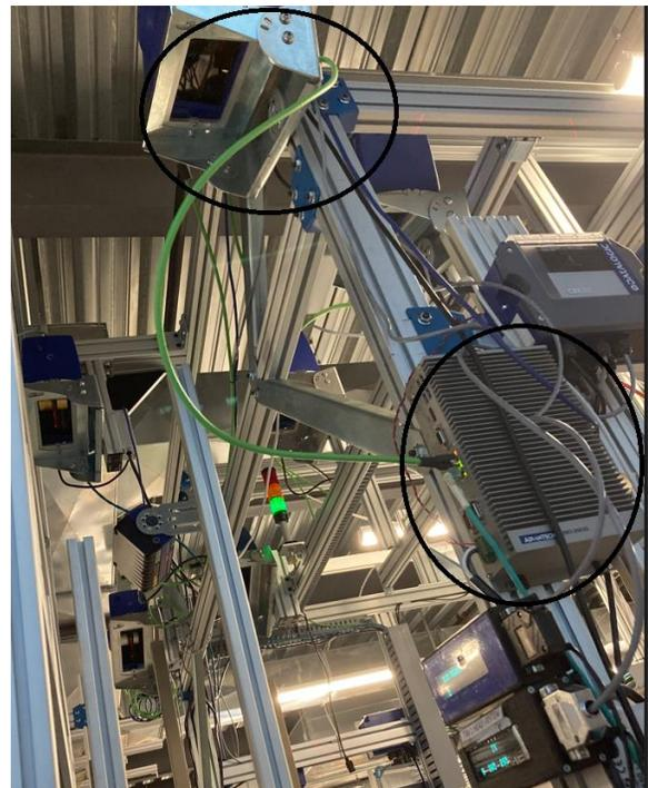
**Location of physical seals for DC3000 (Dimensioning Controller) and the mounting bracket for sensor DM3610-3300 /
