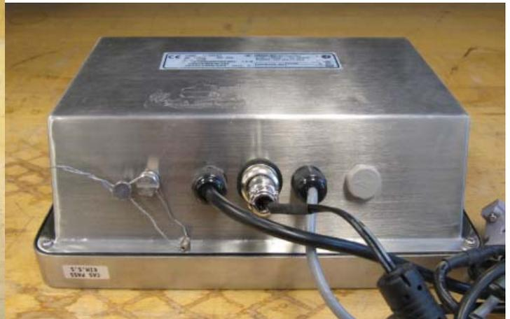
**Typical seal for models CI-200S and CI-200SC / Scellage typique des modèles CI-200S et CI-200SC**
