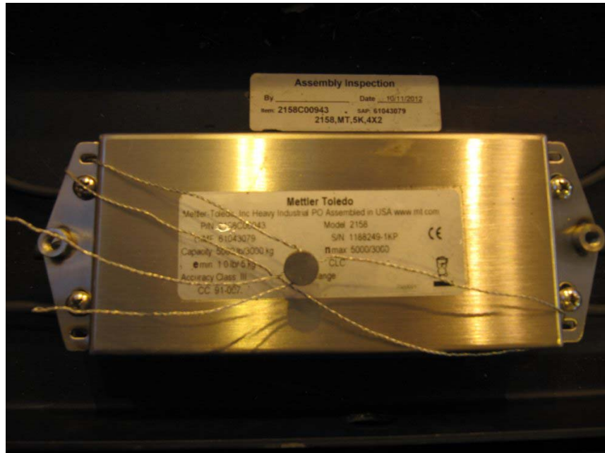
Typical sealing / Scellage typique
