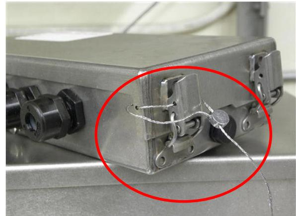
**Typical seal for sectional controller model ACC-2000-1A /
