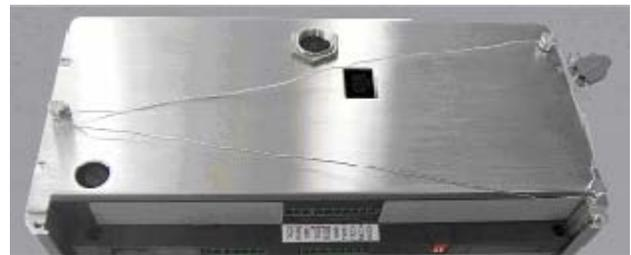
**Typical sealing of the IND560 / Scellage typique de la IND560**
