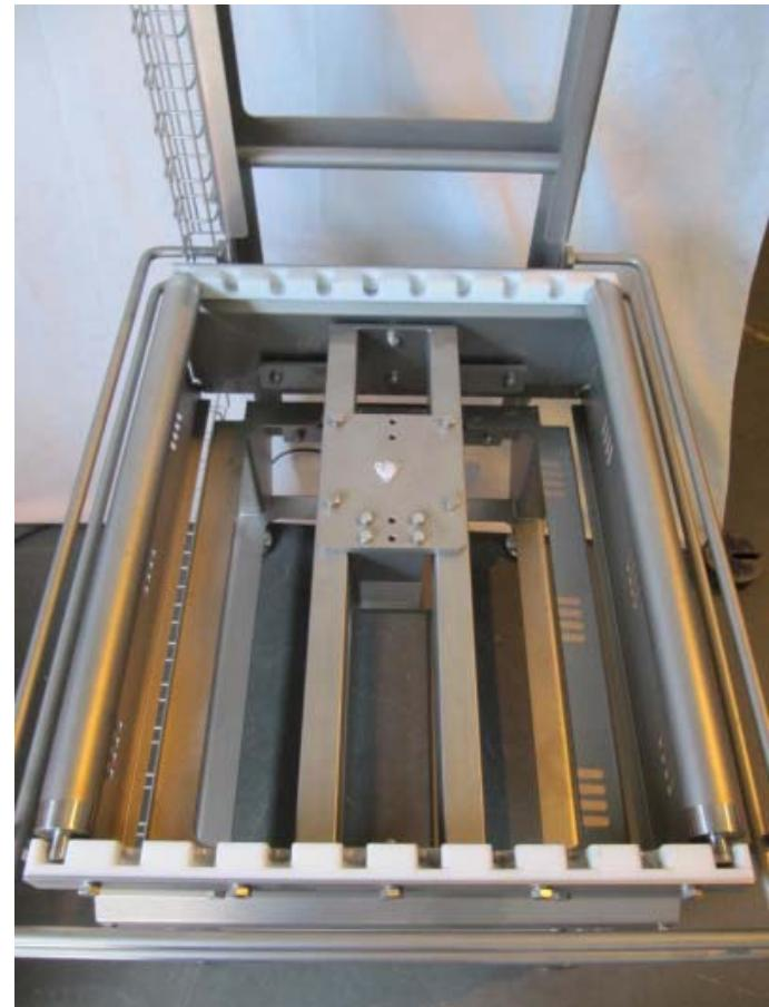
Sub platter and load cell mounting / Sous plateau et
