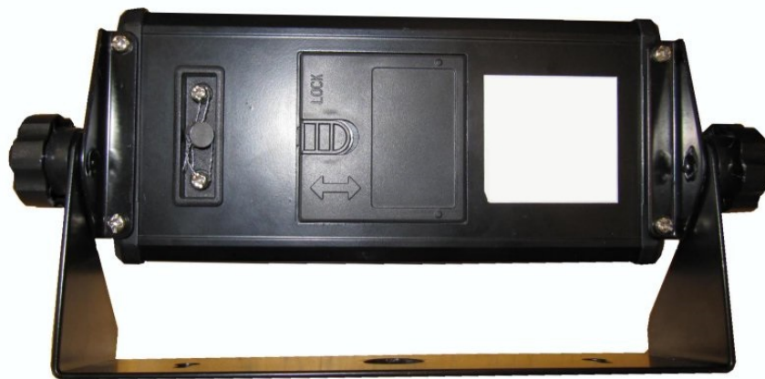
Typical Sealing / Scellage typique
