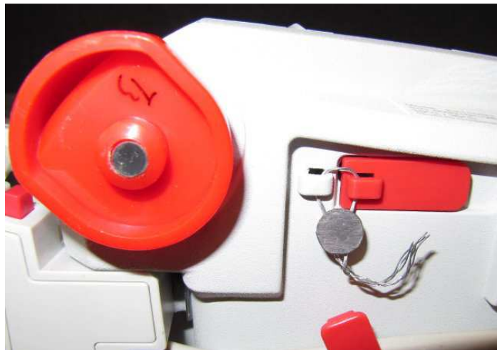
Typical sealing / Scellage typique
