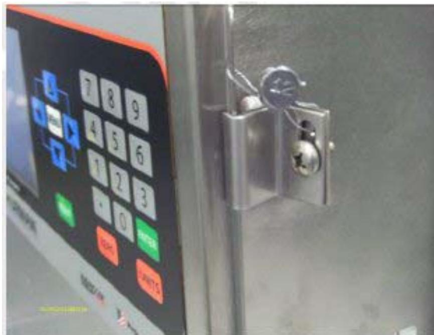
**Typical sealing of models TS-3200-3 and TS-3200-3A / Scellage typiques des modèles TS-3200-3 et TS-3200-3A**
