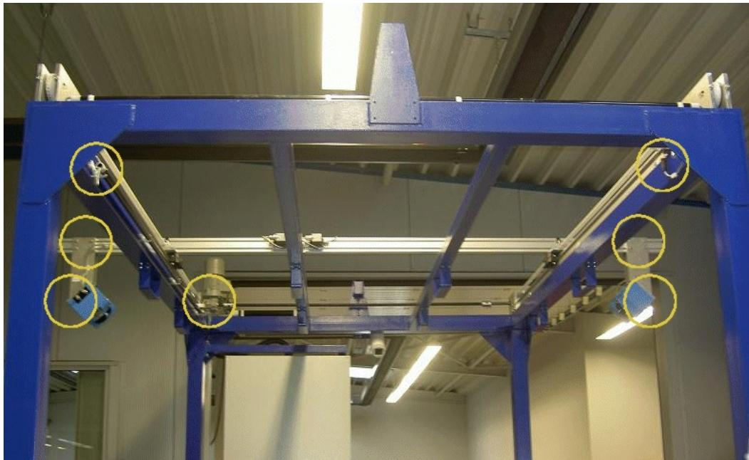
**Sealing locations / Emplacement des scellés**
