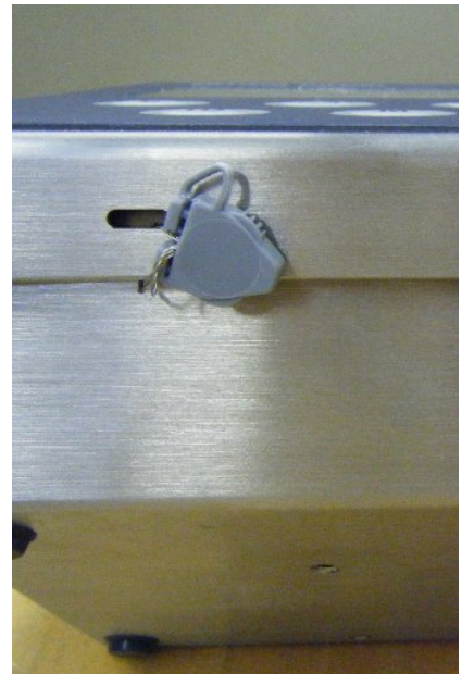
Typical Sealing / Scellage typique
