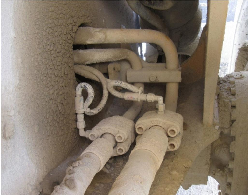
**Typical pressure transducer installation /
