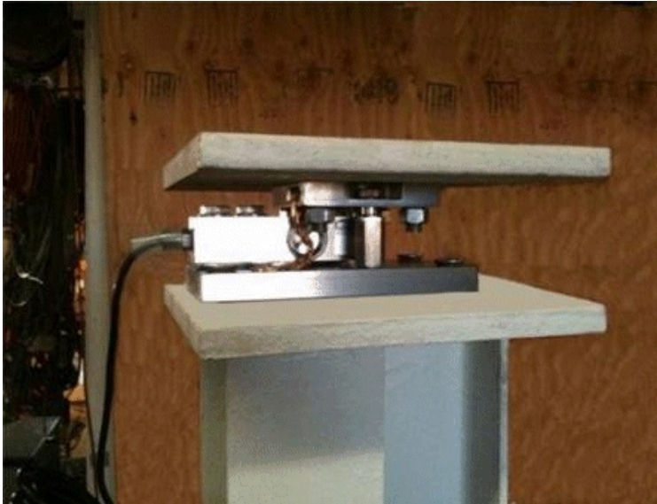
Photograph of typical load cell mounting / Photo du montage typique des cellules de pesage
