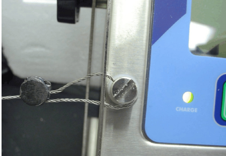
Typical sealing (stainless steel enclosure) / Scellage type (boîtier en acier inoxydable)
